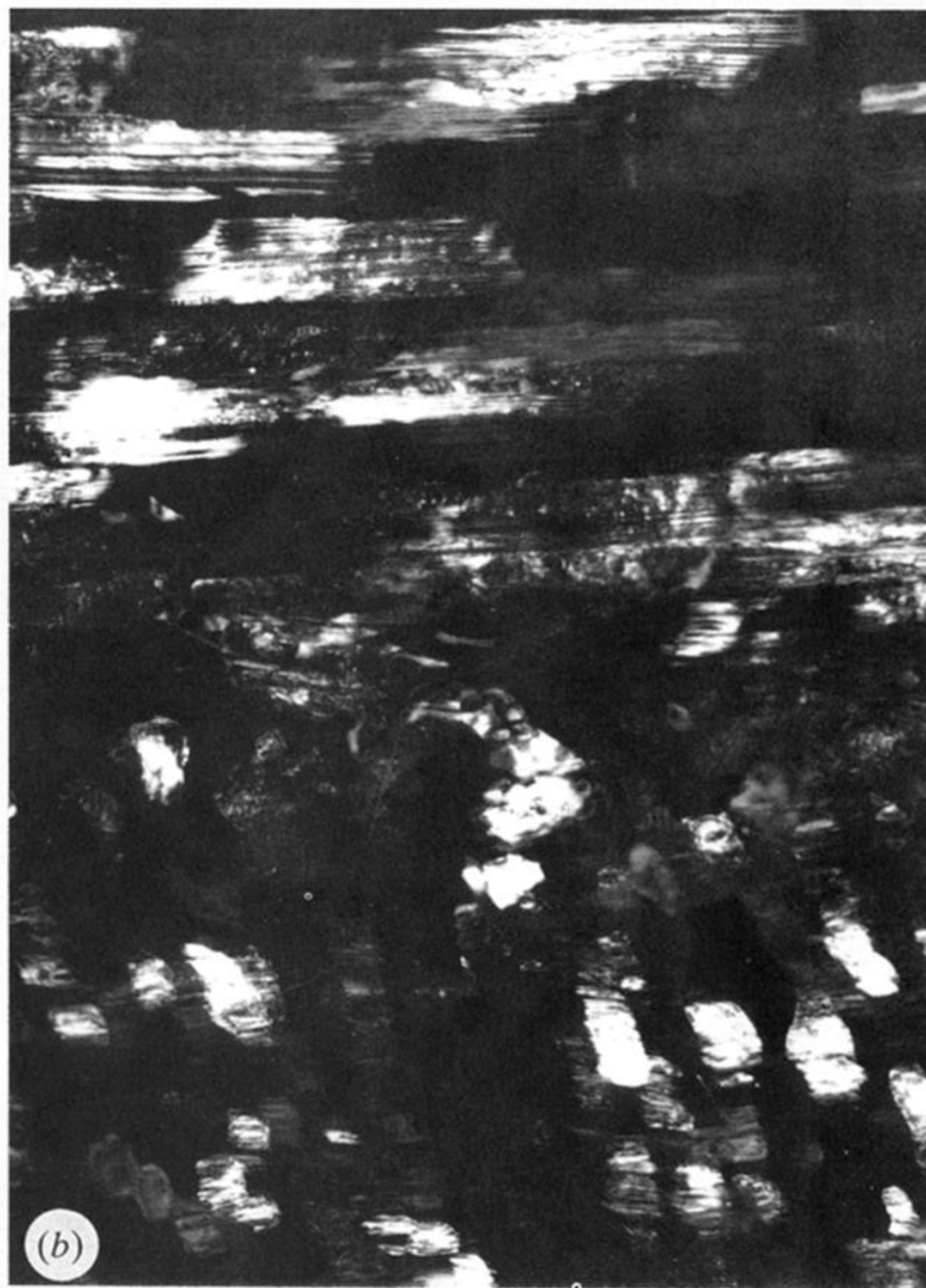
Figure 11. Oliva sayana . (a) Bright field TEM image of first order boundary zone and (inset) superposed selected area diffraction pattern (SAD) from the zone. Note (110) winning and some porosity. (b) Centred dark field TEM image corresponding to (a), recorded with the objective aperture positioned around the almost coincident 112 and 02 reflections (from third order lamellae), as indicated in the inset of (a). (c) [11\bar{1}] zone axis SAD, with minor arcing of reflections, from field near (A) in (a). (d) [22\bar{1}] zone axis SAD, with strong arcing of reflections, from field centred on (B) in (a).
