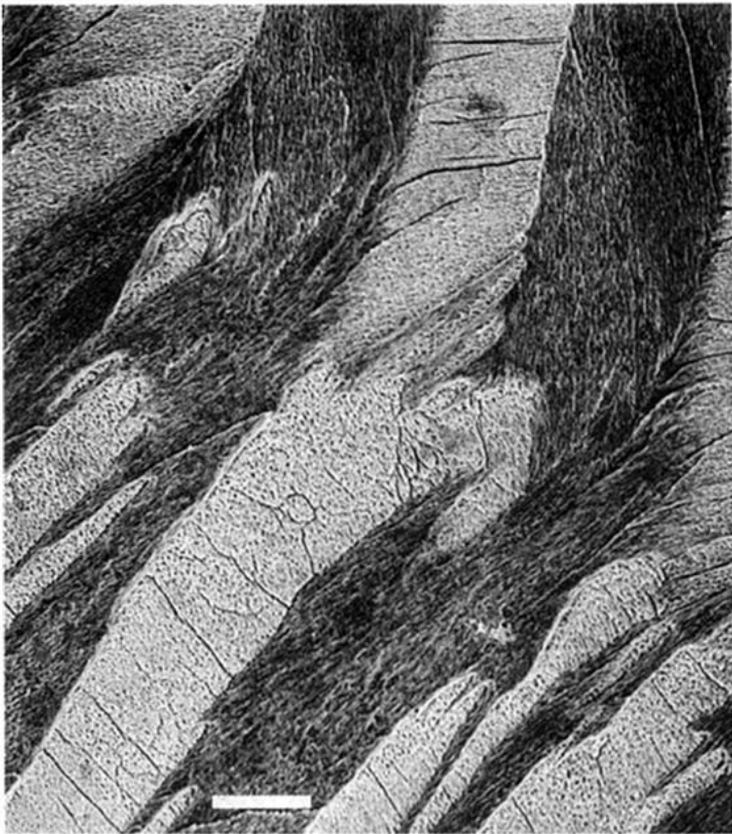
Figure 6. Etched radial section of Conus magus showing the boundary between two xLM layers. Scale bar = 20 \mu\text{m} .
