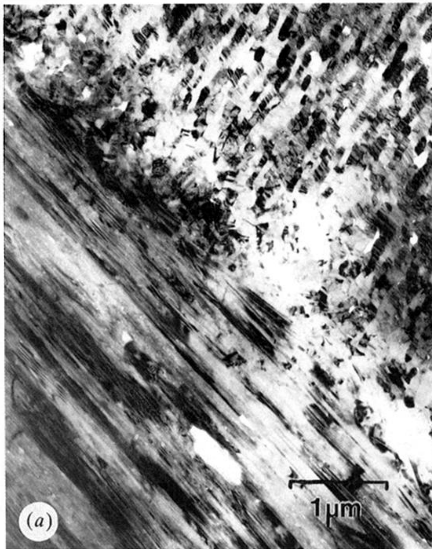
Figure 10. Oliva sayana . (a) TEM image of the boundary zone between first order lamellae, with one set of third order lamellae approximately 'end-on' and the other 'side-on'. Note the approximate parallelism of (1\bar{1}0) twinning across the boundary zone, although a few third order lamellae right at the boundary are strongly misorientated. (b) [31\bar{2}] zone axis diffraction pattern from 'end-on' third order lamellae in (a), showing strong texture.
